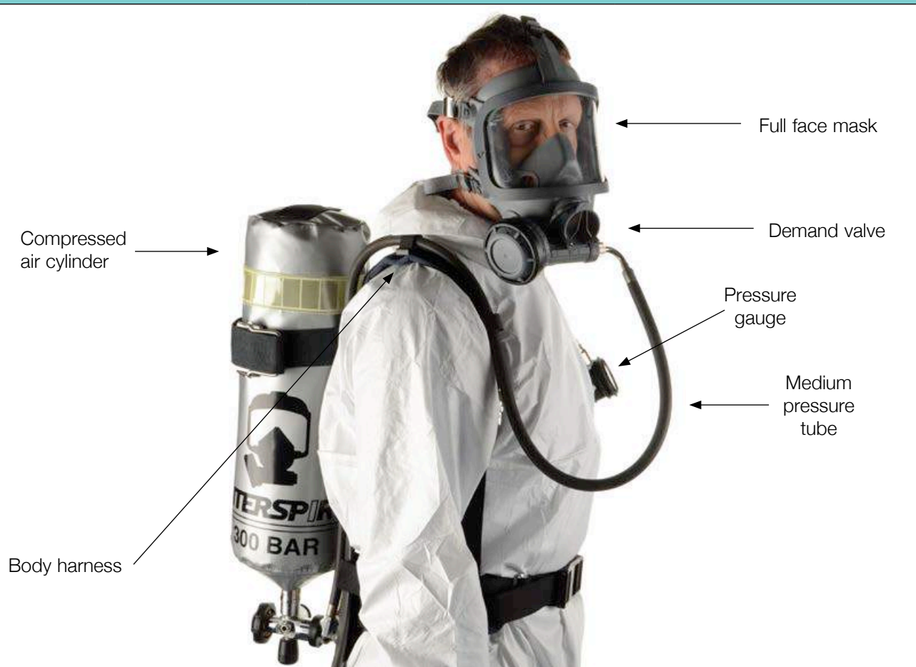
Figure 21 Demand valve breathing apparatus
